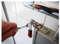
In case the cover does not seal properly anymore, the upper side can be readjusted via the handle of the clamping lever and the lower side via its hinges. This has also an impact on the closing effort.
