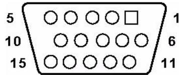
Figure 2.6 VGA Connector
