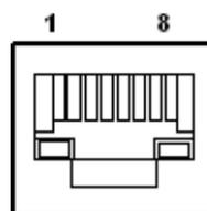
Figure 2.7 Ethernet Connector
