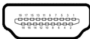
**Figure 2.5 HDMI Connector****Table 2.2: HDMI Connector Pin Assignments**
