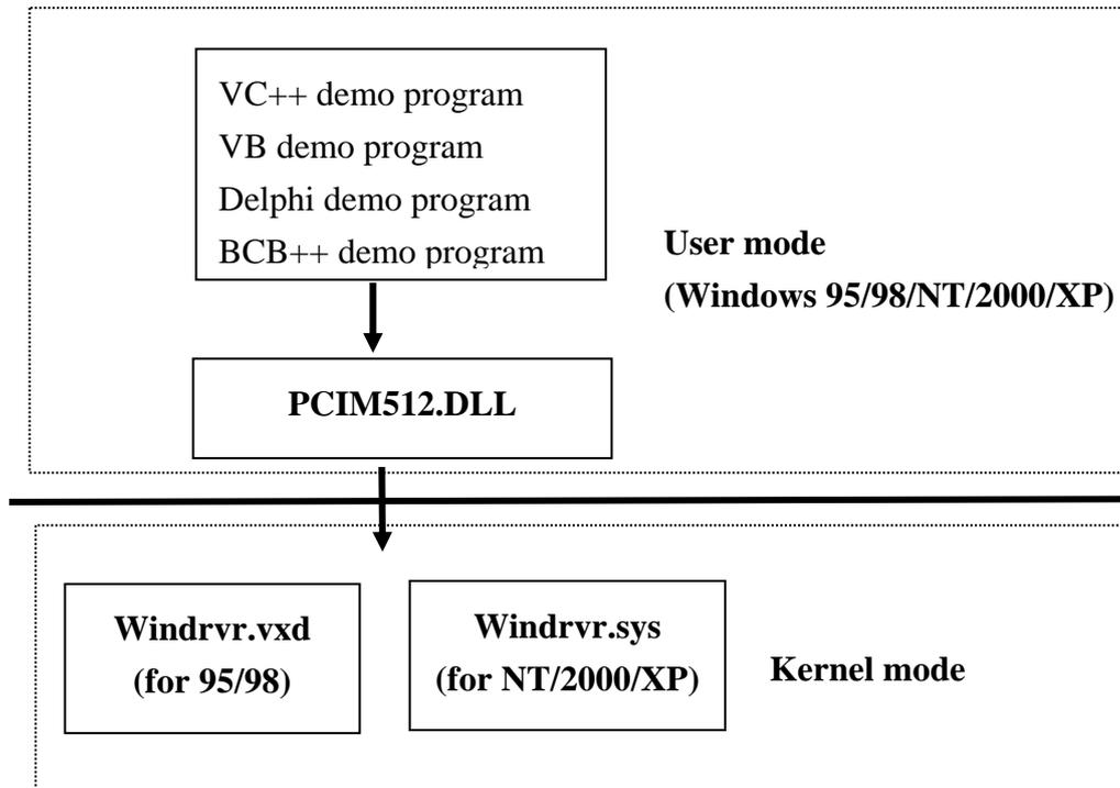
The install shields installs kernel driver and DLL driver system. **All demo program & DLL are the same for 95/98/NT/2000/XP.** However, the kernel driver is different for different system as follows:
