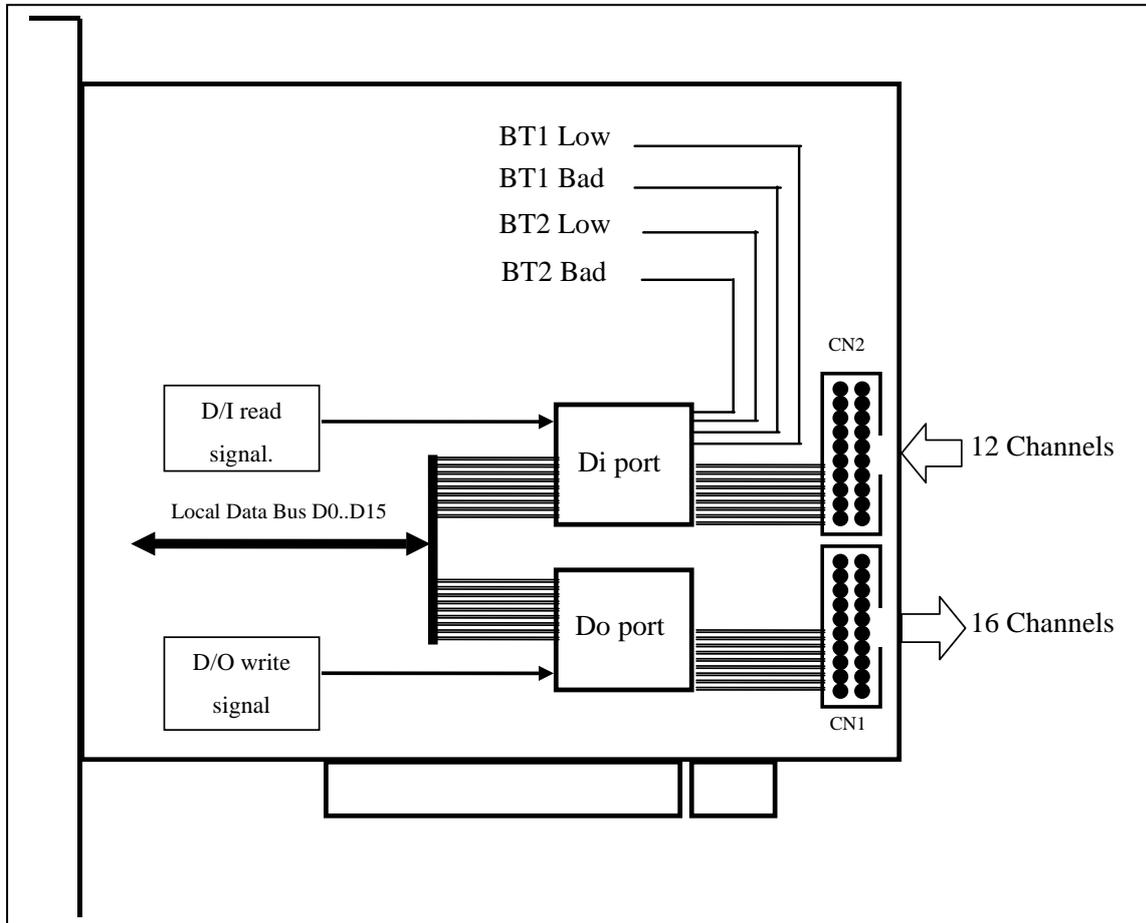
The D/O port can be connected to the DB-16R or DB-24PR. The DB-16R is a 16 channel Relay output board. The DB-24R is a 24 channel Power Relay output board. (note: only 16 channels of these 24 channels are valid).
