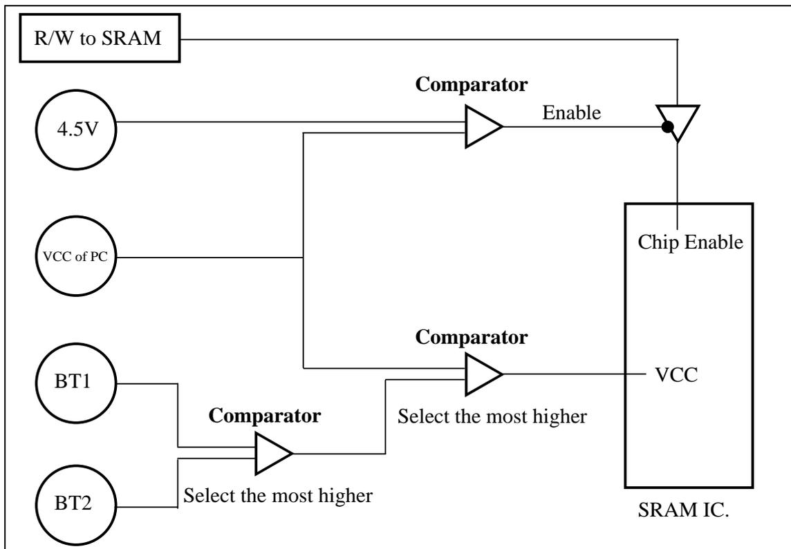
The power supply of SRAM is selected from the highest voltage of PC-VCC, BT1 & BT2. The initial voltage of BT1 & BT2 is about 3V. If the PC is power on, the PC-VCC will be about 5V. If the PC is off, the PC-VCC will be about 0V. So when the PC is power on, the PC-VCC will supply power to SRAM. In this condition, BT1 & BT2 will preserve their battery for later usage.
