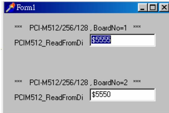
The screenshot shows a Delphi window titled 'Form1' with two sections for D/I/O read results. The top section is for BoardNo=1 and the bottom section is for BoardNo=2. Each section contains a text box for the 'PCIM512\_ReadFromDi' field.
