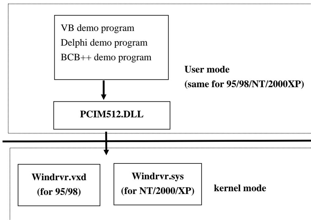
The install shields will install kernel driver, DLL driver & application demo programs to system. **All demo program & DLL are same for 95/98/NT/2000/XP**, but the kernel driver is different for different system as follows:
