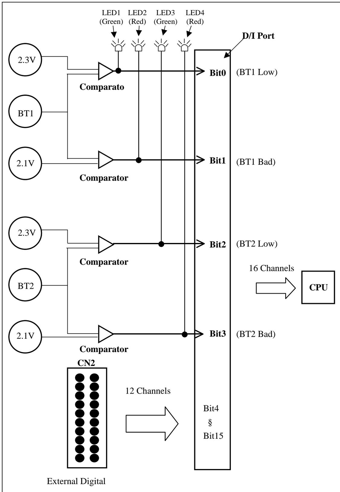
The initial voltage of BT1 will be larger than 3.0V. If this voltage drops to 2.3V, BT1 can still keep the stored data in SRAM for months. **It is recommended to replace both BT1 & BT2 when either BT1 or BT2 drops to 2.3V.** If this voltage drops to 2.1V, the BT1 can still keep the stored data in SRAM for weeks. **You should replace both BT1 & BT2 a.s.a.p. if either BT1 or BT2 drops to 2.1V.**
