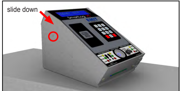
Figure 14. Sliding the SmartLog V5™ into the bracket and securing it into place with the 4-40 screw
