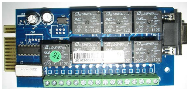
Figure 20: Relay card appearance
