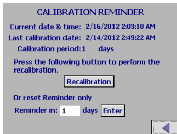
Figure 14 – Calibration Reminder Screen View
