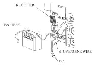
Use 12V and more than 45A·H battery, connect its positive lead to start relay terminal while connect its negative lead to engine mounting screw, base screw or other grounding point with the engine. (See Fig. 2)
