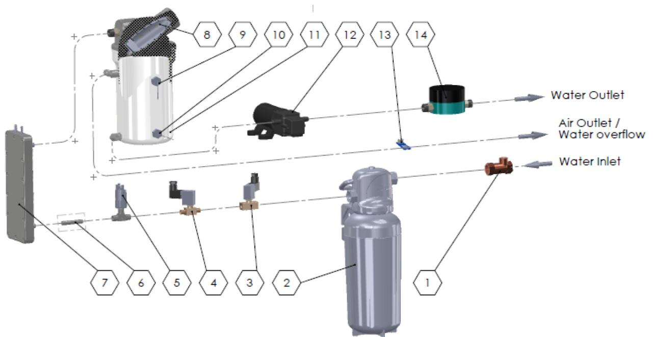
Figure 3-2 Process diagram: 1: DS EN/6117 Approved non-return valve; 2: Head and cartridge for filter/softener; 3 & 4: Solenoid valves; 5: Pressure switch; 6: Optional flow restriction; 7: BacTerminator disinfection chamber; 8: Bio Reaction Zone; 9: Water tank with 20mm air gap; 10: Level sensors; 11: Pump; 12: Pulsation dampener; 13: Leak detector
