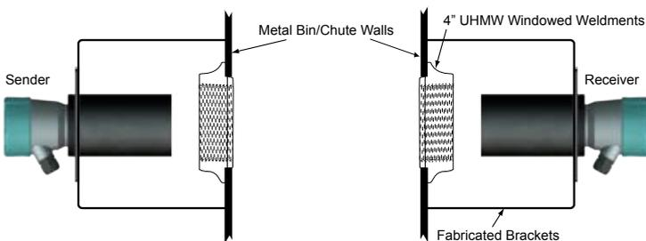
Adjustable microwave mounting bracket welded to vessel wall. UHMW or Teflon Window.
