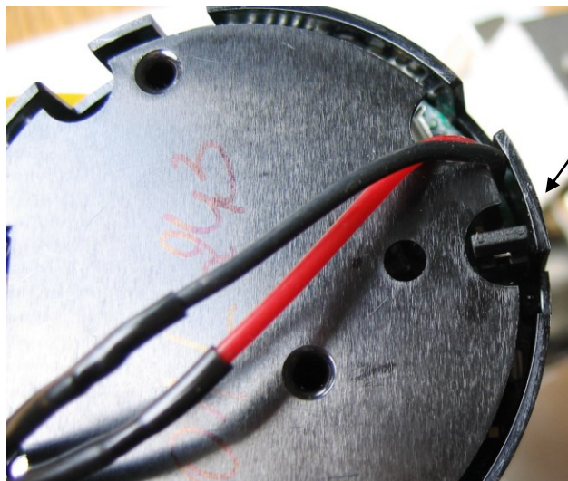
Fig.5. Back lighting jumper view at transmitter electric board (unit display back side).
