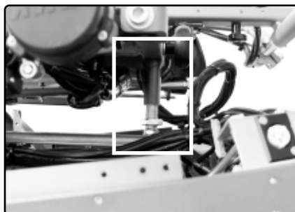
Fig. 7. The seat support is fitted so it provides support for the rear of the seat frame
