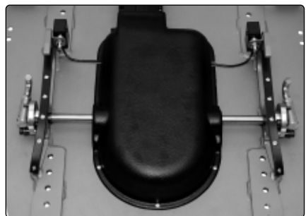
Fig. 3. Fitting of the cover for electric locking.
