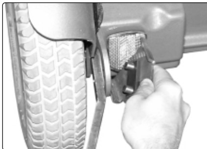
Fig. 1. Guide plate and spacer plate
