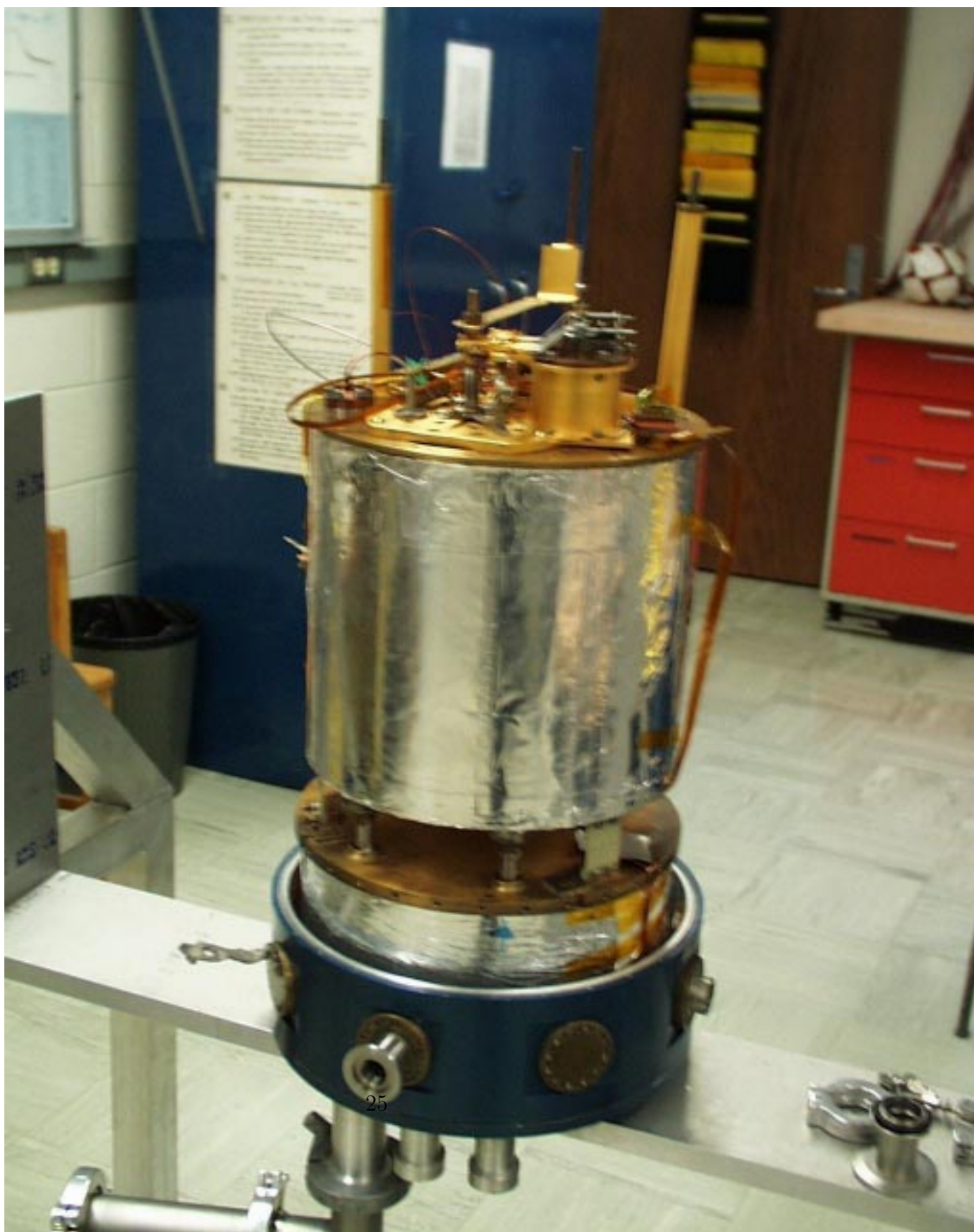
Figure 3.2: The open dewar. Shown is the coldplate which is the top of the liquid helium tank. Below it is the liquid nitrogen tank
