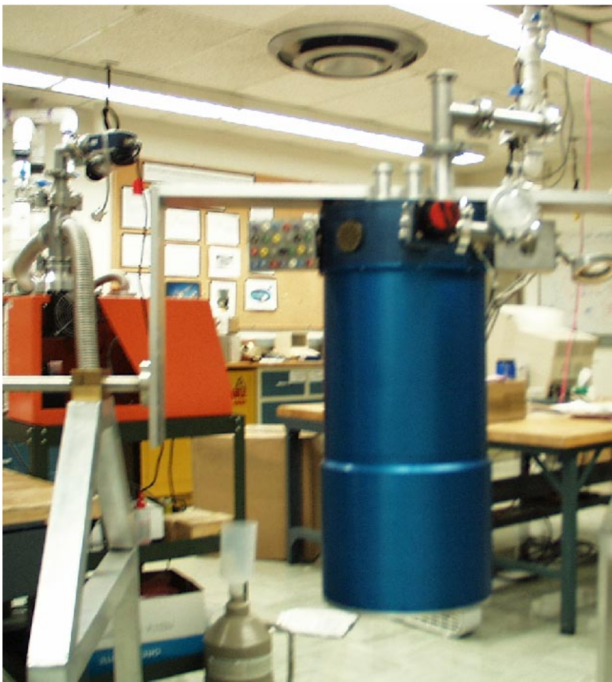
Figure 3.1: The dewar when it is put together and closed up.
