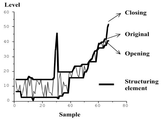
The opening eliminates peaks that are thinner than the structural element. By choosing an appropriate size of radius R the opening separates background signal from relevant one. Indeed, thin background peaks are eliminated, but in return
