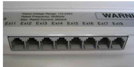
Fig 2: The 8 RJ12 extension ports of the Premier PABX
