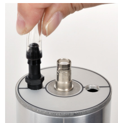
Attach air hose to one fitting
