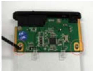
2. Slide the hard drive into the enclosure and use the remaining screws to shut the enclosure.
