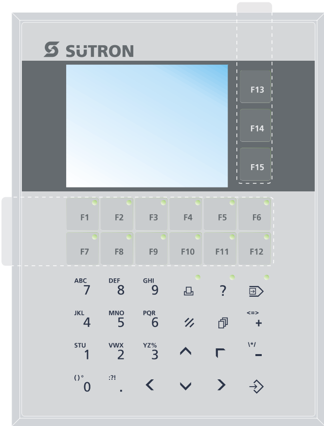
Figure 3-5 Position of the slide-in identification strips at BTM07AM
