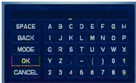
**Note:** While changing the name of a sub user, on screen keyboard will be available as shown on the left. Press MODE to toggle between different sets of characters.
