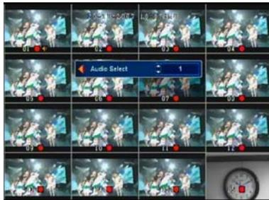
**H.264 DVR** allows recording audio per each channel of video inputs, and audio outputs are available for only one selected channel at a time. In order to select an audio channel for audio output, press **FUNC** (ALT) and then **MENU** on the front panel (F1) and then **MENU** on the remote controller). It will allow the user to select an audio channel between 0 and 16 or Mute to turn off the audio.
