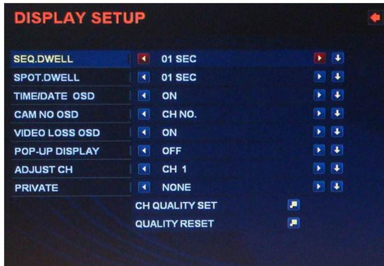
1. **SEQ.DWELL** Select dwell time between 1 to 60 seconds for the switching interval under sequential display mode. Press Left/Right Direction buttons to decrease/increase dwelling time.
