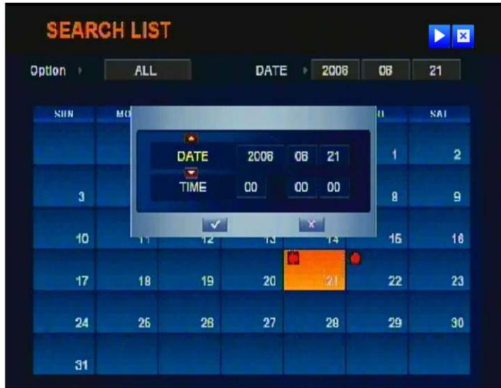
From the above screen, press **COPY** on the Front Panel and **USB** button on the remote controller. “START” and “END” will be prompted to set date and time to backup, in order of year, month, day, hour, minute and second. Set desired time range, move to the check mark, and press **ENTER**.
