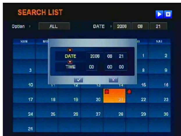
The user is able to select specific date and time to start playback. Once the date and time are selected, press **ENTER** to playback from that moment. Refer to **6-4.Playback** for detail instruction on playback.
