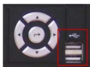
These 2 USB Connectors can be used for a mouse and a USB Memory device. Device(s) will be automatically detected upon connection.
