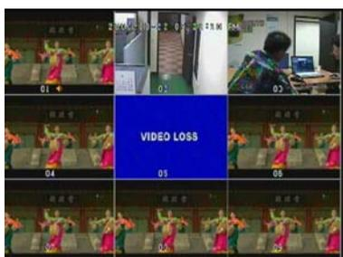
Display 9 video channels at a time, starting from Ch. 1 ~ 9. By pressing this button repeatedly, the display will toggle between Ch.1 ~ 9 and Ch.8 ~ 16.
