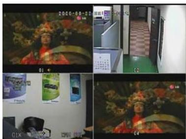
Display 4 video channels at a time, starting from Ch. 1 ~ 4. By pressing the quad button repeatedly, the display will rotate from Ch. 5 ~ 8 to Ch. 9 ~ 12, Ch. 13 ~ 16, and then back to Ch. 1 ~ 4 so on and so forth.
