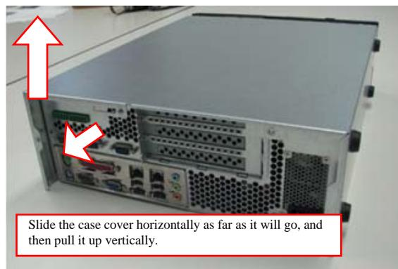
Figure 3.1 Removing the top cover
