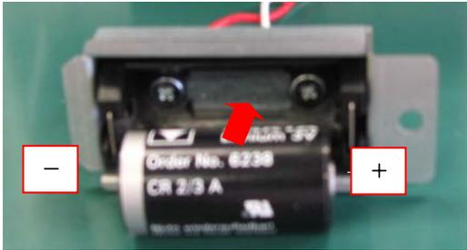
Confirm the positive poles and negative poles, and insert the battery.
