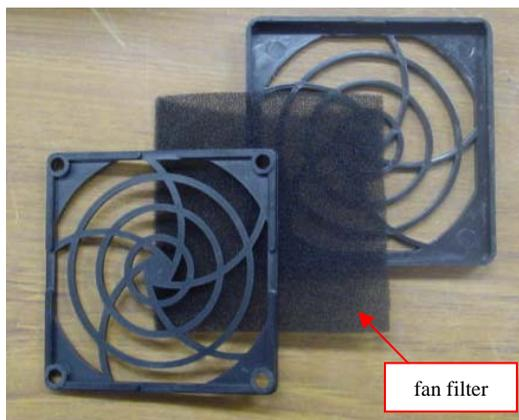
**Figure 3.12 Remove the fan filter**
