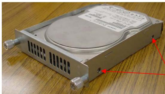
Tighten inch flat head screw from the side of 3.5inch bay ( four in total including the other side)
