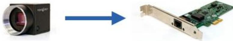
Figure 8. Single camera connected directly to a host adaptor
