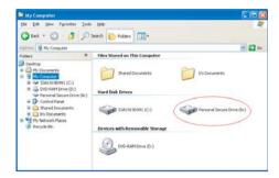
In this screen, although the Personal Secure Drive has been detected as Drive [N:] with a drive name of Personal Secure Drive, it is possible to change this setting in the User Settings of the Infineon Security Platform Settings Tool.
