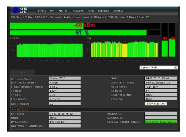
While sharing the same information as the Base Station the CPE Unit also has the received signal level in dBm, the Tx CCQ (Client Connection Quality) in % and the individual Rx levels for the two MIMO chains (Chain0 and Chain1) in dBm.
