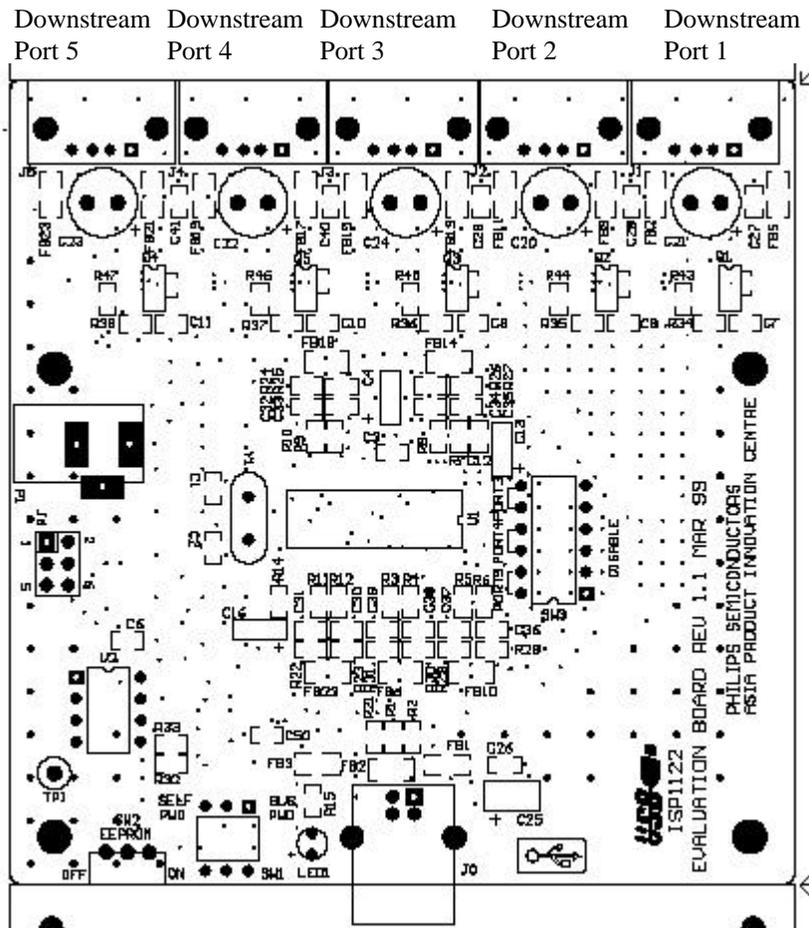
Figure 2 Component Placement of the ISP1122 Demo Board
