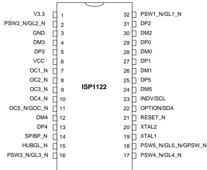
**Figure 1 Pin Diagram of ISP1122**
