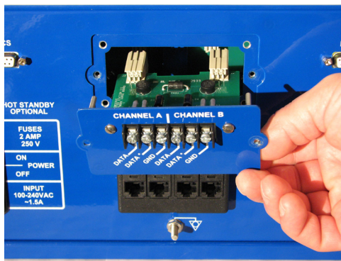
Figure 11.8 - Removing Network Surge Protector
