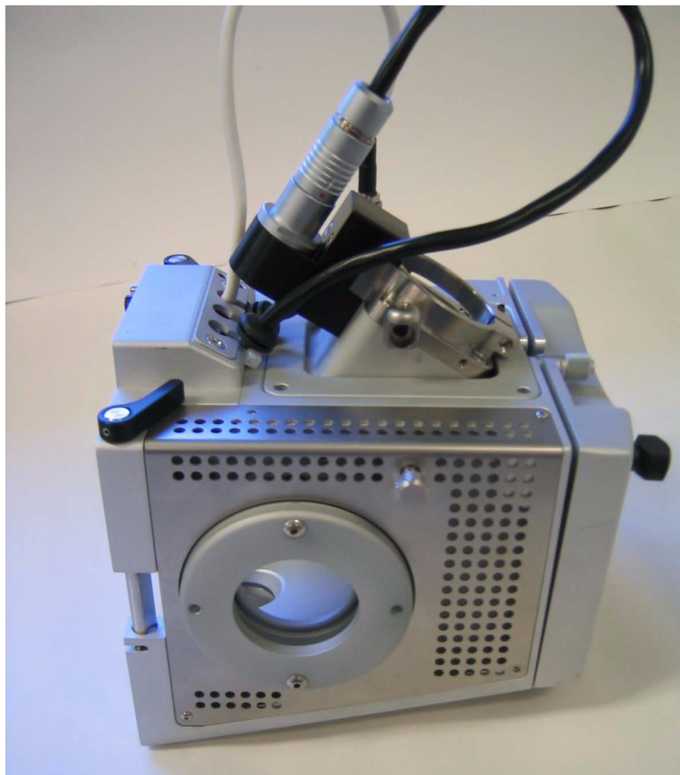
Figure 56. Completed APPI adapter ring installation
