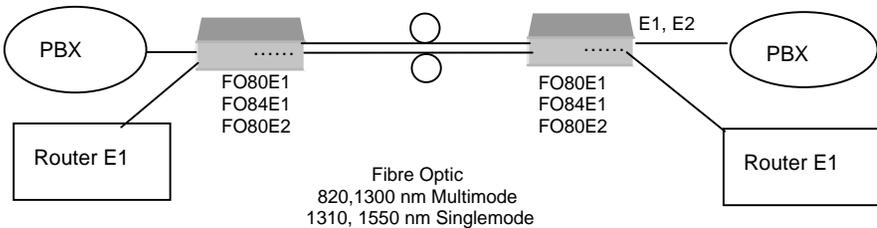
With a FO80E2 local, the remote modem can be another FO80E2 or an FO8011 in transparent mode. The release software must be identical. Speed at 8448 or 2048 KBPS.
