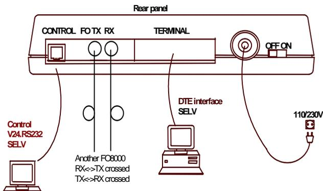
(\*) 110/230VAC / 5Vdc wallmount power supply or 110/230VAC or 48 Vdc cable as applicable.
