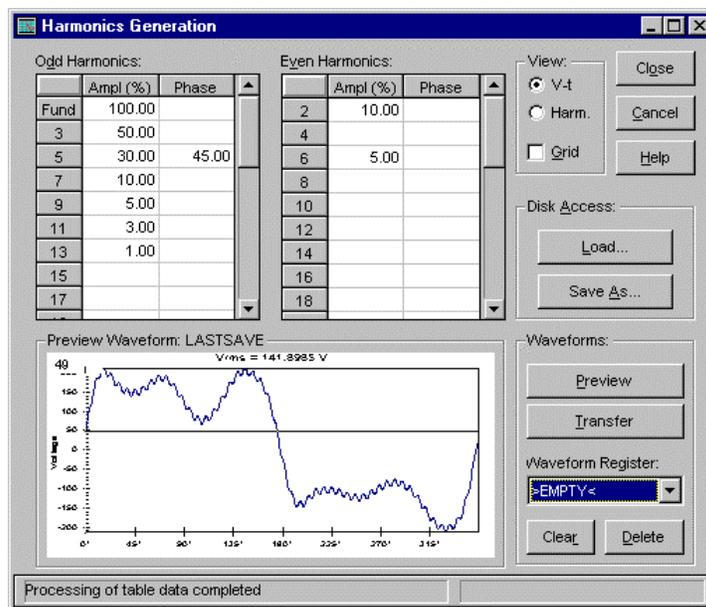
Figure 4-8: Custom Waveform Creation with GUI Program
