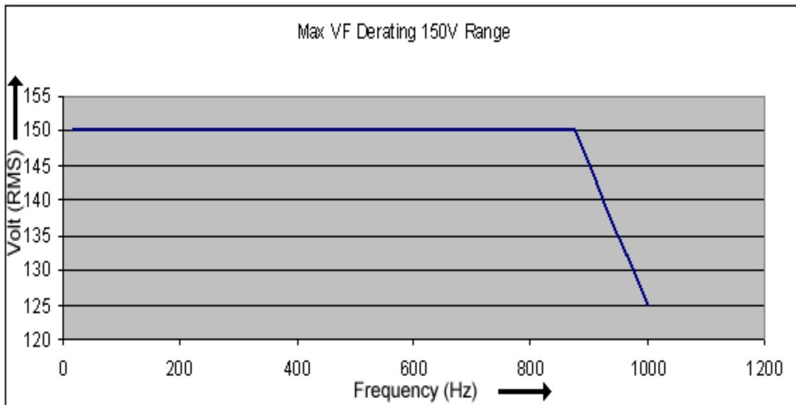
Figure 2-8: -HF Option Voltage Frequency Rating 150V range
