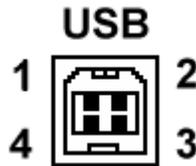
Figure 3-13: USB Connector pin orientation.
