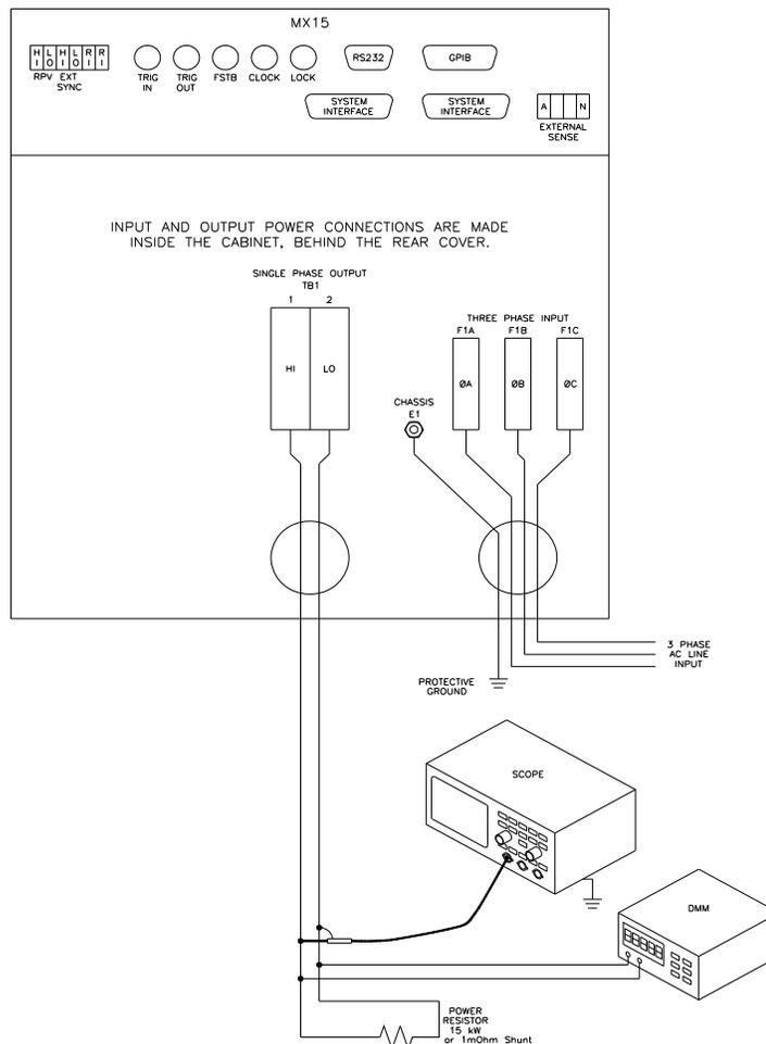
Figure 6-1: Calibration Setup MX45-1 (Rear view)
