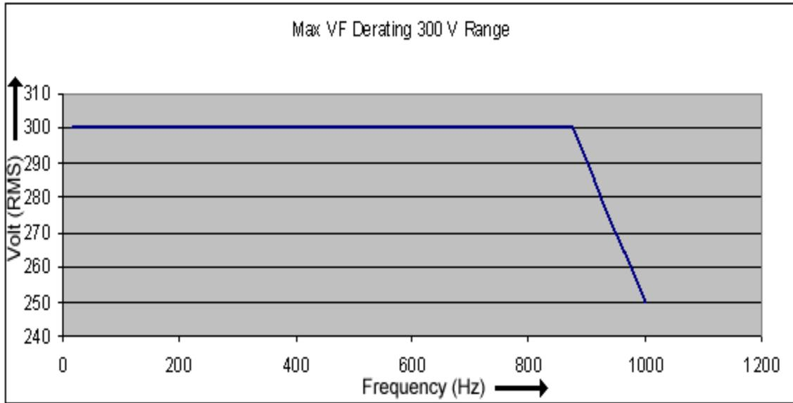
Figure 2-7: -HF Option Voltage Frequency Rating 300V range
