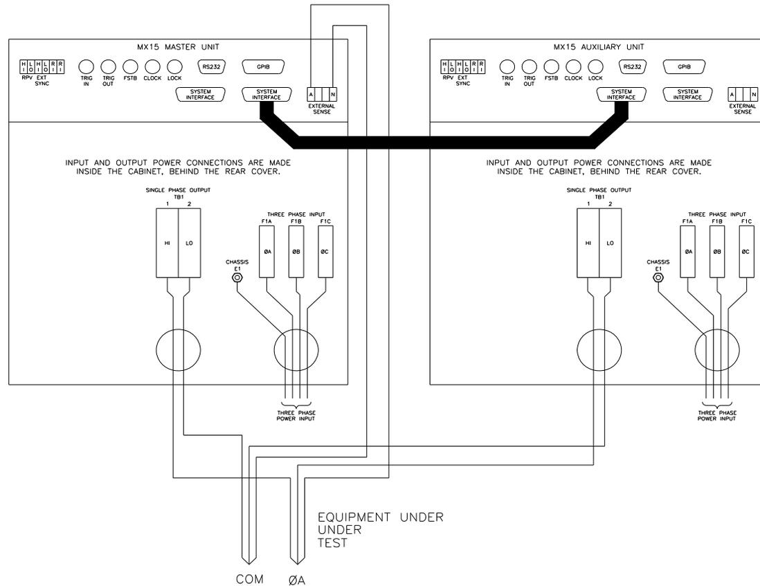
Figure 3-7: MX30/2 or MX30/2-MB Output Wiring (Rear view)
