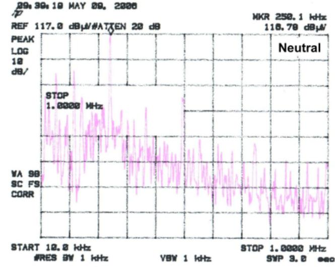
Figure 2-10: MX45 Output Noise 10 KHz – 1 MHz
