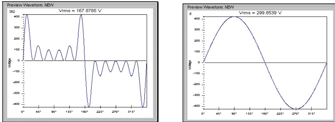
Figure 4-9: Waveform Crest Factor Affects Max. rms Voltage
