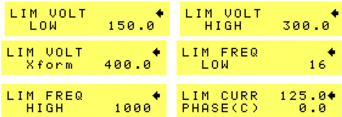
The Limit menu displays the maximum available value for voltage, frequency and current range of the power supply. This screen is used for information only and contains no user changeable fields. The limit values shown cannot be changed.
