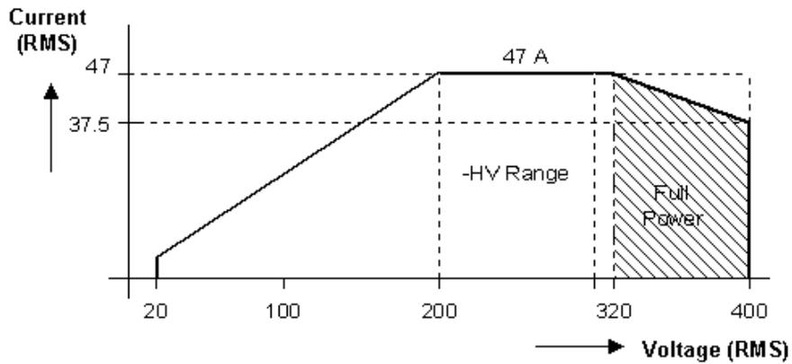
Figure 2-6: Voltage / Current Rating Chart, -HV Option – Derated.
