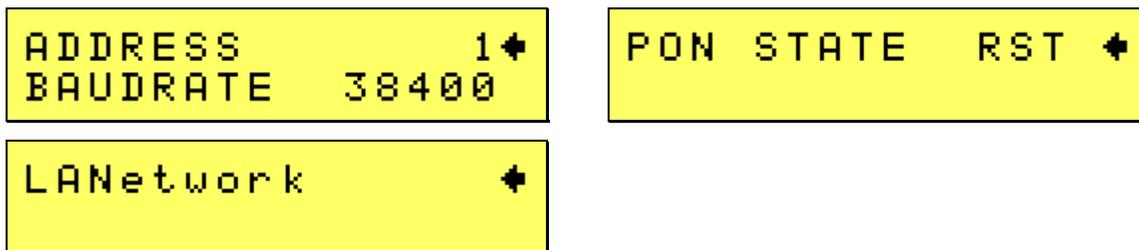
The configuration menu may be used to configure various aspects of the instrument such as the serial port (including USB and LAN), IEEE-488/GPIB address and the power-on settings of the supply.
