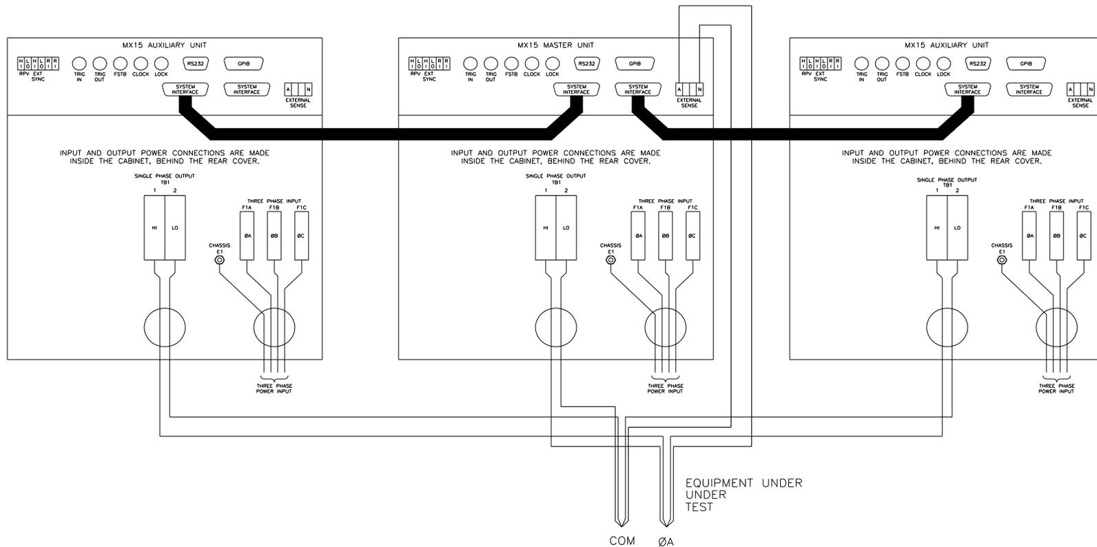
Figure 3-9: MX45/3 or MX45/3-MB Output Wiring (Rear view)
