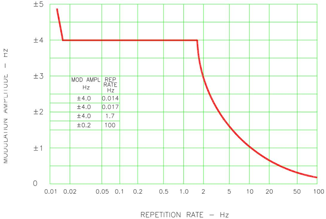
Figure 9-5: Frequency Modulation
