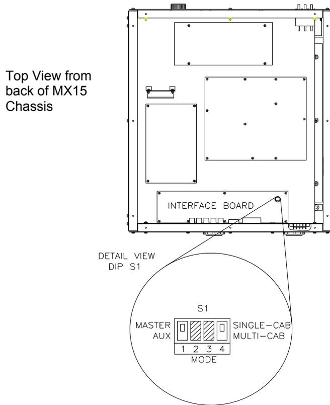
Figure 3-14: Multi-Cabinet DIP Switch Location and Setting
