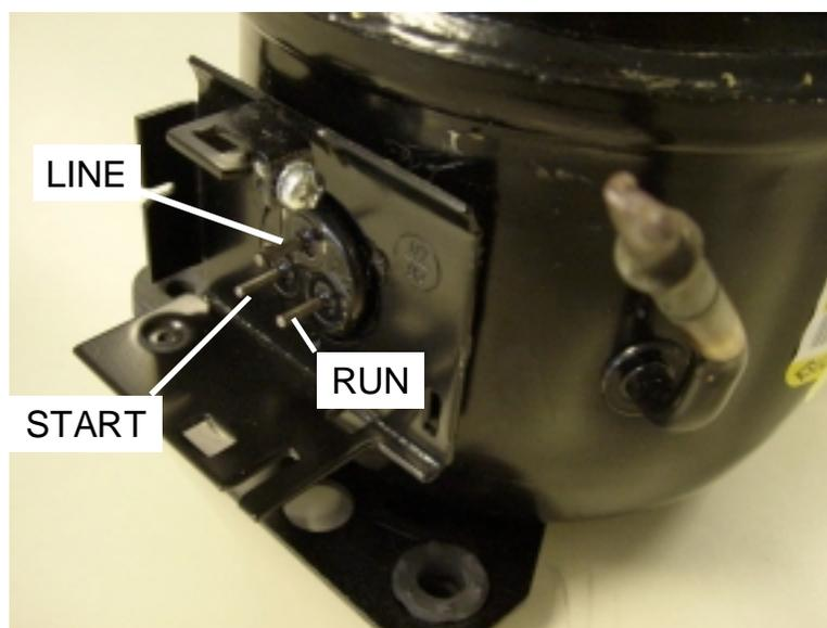
Often, compressor motors are used with a starter that includes a thermal protection against excessively high currents or overheating. This protection is called a "klixon", and is shown in Figure 7. When you are using the THERM01EVAL board its better to keep this starter, in order to let the klixon work. In this case, the motor connections can still be accessible, this depends on the starter model, as shown in Figure 7.
