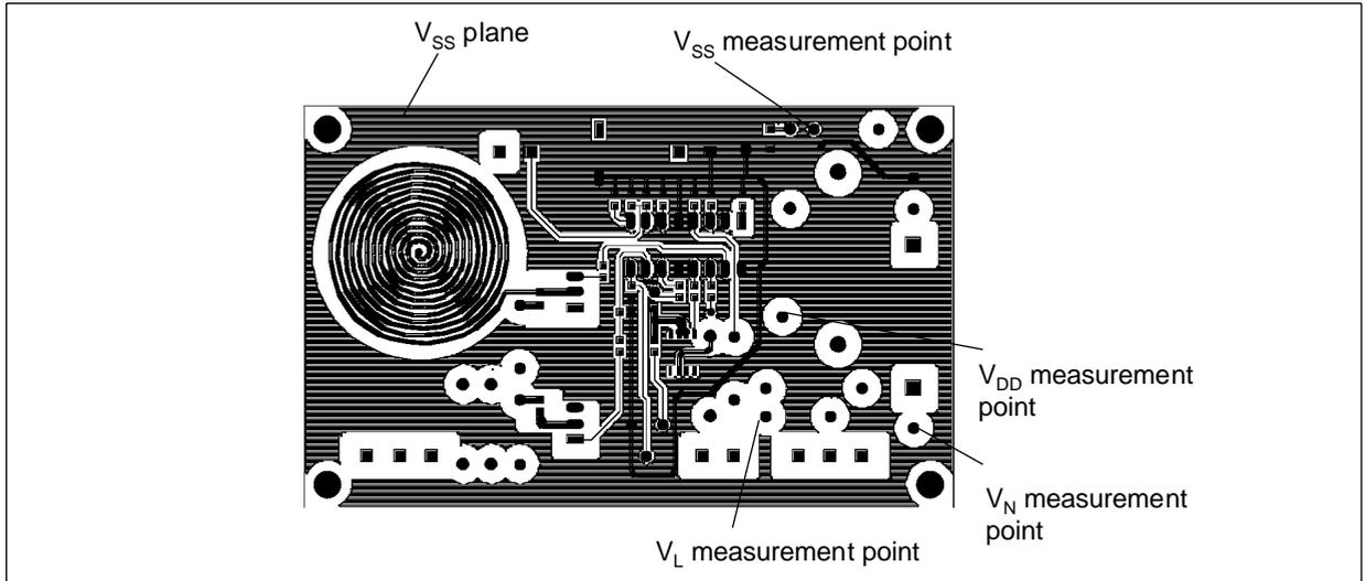
Figure 4. Bottom layer view (from component side)
