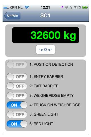
The top part will show the actual weight and a button to zero the scale. Depending on the setup of the UniWin solutions, the zero may only be activated for some users, or only when a weight is within the so-called zero range.
