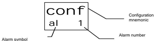
A 4-digit code is displayed on the upper display, with the current configuration of the Alarm no:
