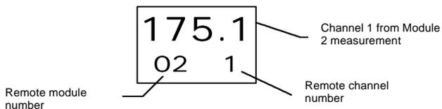
Press the **Function** key consecutively, and the channel number and the value of its measurement will be displayed. After channel 8, the **ALAr** and **PASS** parameters appear, beginning again with channel 1.
