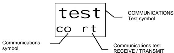
The Communication Test will appear. If a communications link is established, the symbols **⌈** (RECEIVE) and **⌋** (TRANSMIT) will be
