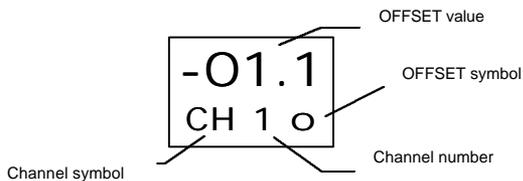
Press the **Shift** and **Increment** keys to enter the required Offset value. Once the data is entered, press the **Validation** key.
