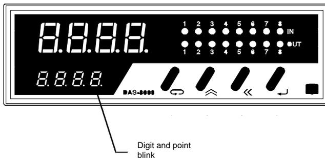
Once proper operation of all display elements has been checked, press the **Enter** or the **Function** key to exit the display test.
