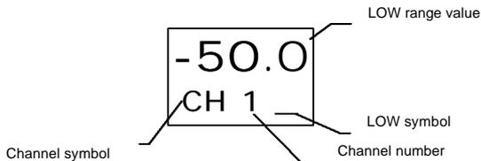
Enter with the **Increment** and **Shift** keys the new low range value, and press **Validation**.
