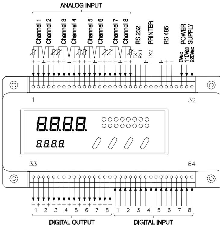
In the upper row, there are analog inputs connections consisting of 8 blocks of two terminals (+ and -) for mV or mA with shunt, sharing a third terminal, centered between every two channels, for line compensation in Pt-100 inputs.
