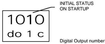
This digit allows you to configure the Initial Status when the device is started up (after a power failure). The possible values are:
