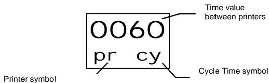
Use the **Shift** and **Increment** keys to modify the value. You can select between 1 and 9999 seconds (if it is configured with a value of 0, this function is deactivated).
