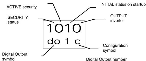
Press the **Shift** key to select the digit that you wish to modify. Each digit of that code represents a configuration parameter of the Digital Output, with the value of the digit representing the possibilities that this parameter can have. Select each one of them based on the configuration desired that is explained in the following sub-sections:
