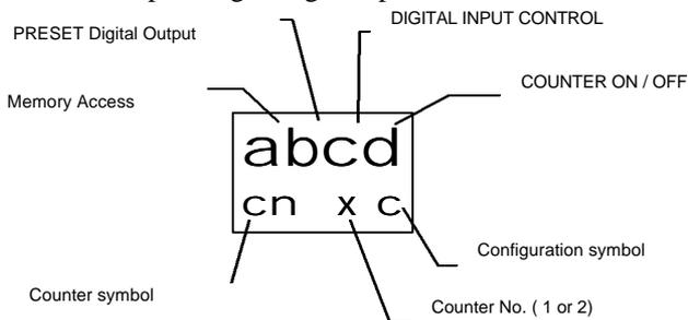
Press the **Shift** key to choose the parameter to be changed and the **Increment** key to choose the data shown below:
