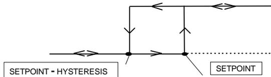
In the **Maximum** type, the alarm is deactivated while the value of the measurement is rising and below the **Set-point**. When it reaches the Set-point, it is activated, deactivating itself when the measurement goes below **Set-point - Hysteresis**.
