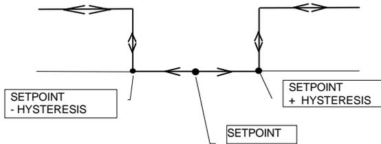
On **Inverted Window** mode the alarm is activated while the measurement value is within the margin set point  $\pm$  hysteresis. Out of this margin the alarm remains deactivated
