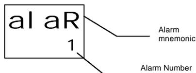
The number of the last alarm will be displayed blinking. Select with the **Increment** key the alarm number that you wish to display and/or modify.
