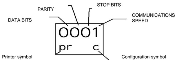
Press the **Shift** key to choose the parameter to be modified, and the **Increment** key to select the following values:
