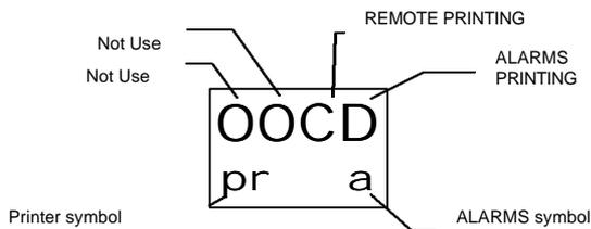
Use the **Shift** key to select the digit to be changed. Each digit of this code represents a parameter for printing alarms and/or remote printing of the measurements, where the digit value is a number representing the several choices of this parameter.
