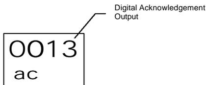
This digit allows the Digital Output number to be selected that will be used for alarm acknowledgement output.
