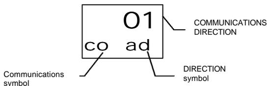
The Communications address no. assigned during the last configuration will be displayed. Use the **Shift** and **Increment** keys to enter the new address no.
