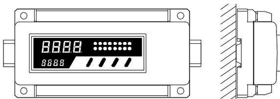
Observe the DIN rail anchorage system of the DAS-8000. You can see that a retractable bolt exists, that is accessible from the outside, visible from the front on the lower part of the DAS-8000 module.
