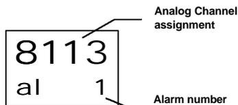
This digit allows you to select the Analog Channel no. that will be linked to the Alarm Number being configured.
