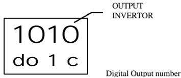
This digit allows you to configure the **Direct** or **Inverse** action of the **Digital Output** regarding the status of the **Alarm** or of the **Remote Action**. The possible values are:
