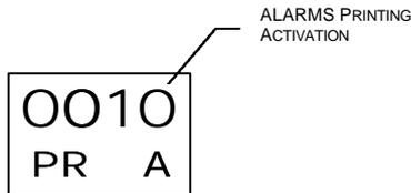
This digit allows to turn alarm printing to be turned On or Off.
