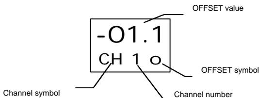
The value that is entered in this parameter, will be added or subtracted (based on the sign that has been given it), to the value of the measurement in all the range.
