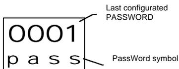
The access password allows the use of 10 digits, 0 to 9, and the letters A, B, C, D, E and F, in any combination.
