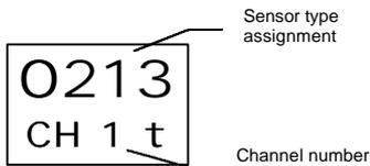
This digit selects the type of Sensor to be adapted to the Analog Channel no. being configured. The possible values are:
