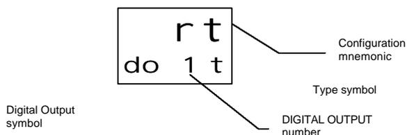
Select by means of the **Increment** key the type of Digital output desired. Once selected, press the **Validation** key.
