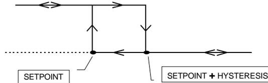
In the **Minimum** type, the alarm is activated while the value of the measurement is rising and it is below the limit of **Set-point + Hysteresis**. When it reaches this value it becomes inactive, and is reactivated when the measurement goes below the **Set-point**.
