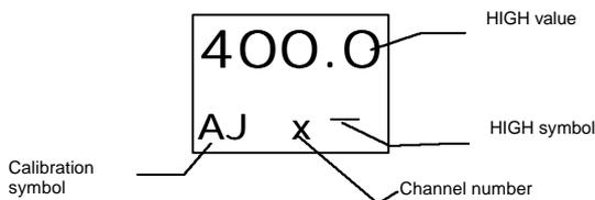
Enter via the terminals corresponding to the channel no., the signal of the high value: 247.05 Ohms (400.0° C of Pt-100).
