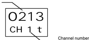
This digit activates or deactivates the Peak Filter signal and also enables the display of the **UNDE** and **OVER** messages when the range is exceeded.
