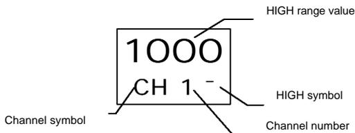
In a signal 4-20 mA with a range of -500 a +1000 mm H<sub>2</sub>O, the low range will be -500 and the high +1000 (does not need exterior Reference of signal or Calibration).
