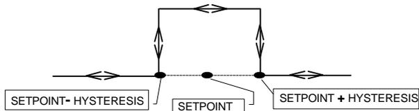
In the **Window** type, the alarm is inactive while the value of the measurement is below **Set-point - Hysteresis** and above **Set-point + Hysteresis**. Inside this margin, the alarm is activated.
