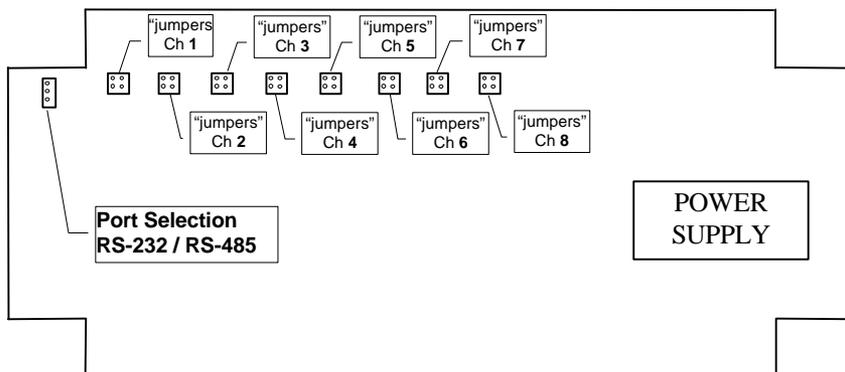
Each of the 8 channels has one disconnectable, black jumper, that should be connected according to the type of sensor used, as indicated in the following figure:
