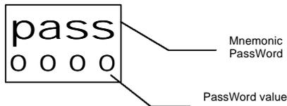
“0000” will appear on the lower display with the right digit blinking. Enter the access password with the **Increment** and **Shift** keys, and press the **Validation** key.
