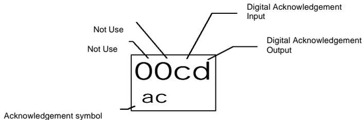
Use the **Shift** key to select the digit to be changed. Each digit of this code represents an Alarm Acknowledgement Parameter, where the digit value is a number representing one of several choices allowed by the parameter.
