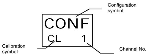
Select with the **Increment key** the maladjusted channel, and without needing any external signal generator, press 3 times, consecutively and quickly, the **Shift key**.
