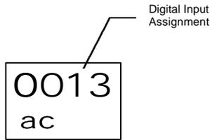
This digit allows the Digital Input number to be used as a digital alarm acknowledgement input.
