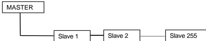
The Master module generates the request messages, while the Slave provides the answer to these requests. You must keep in mind that only the Master can initiate the exchange of messages.
