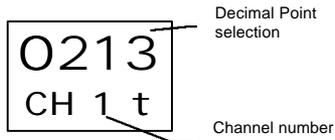
This digit allows you to assign the decimals of the range associated with the Analog Channel no. being configured.
