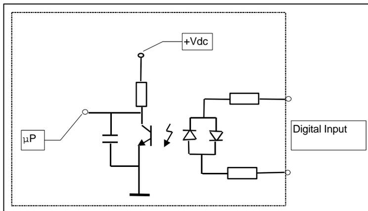
NOTE: The input impedance is approximately 12 K $\Omega$ .
