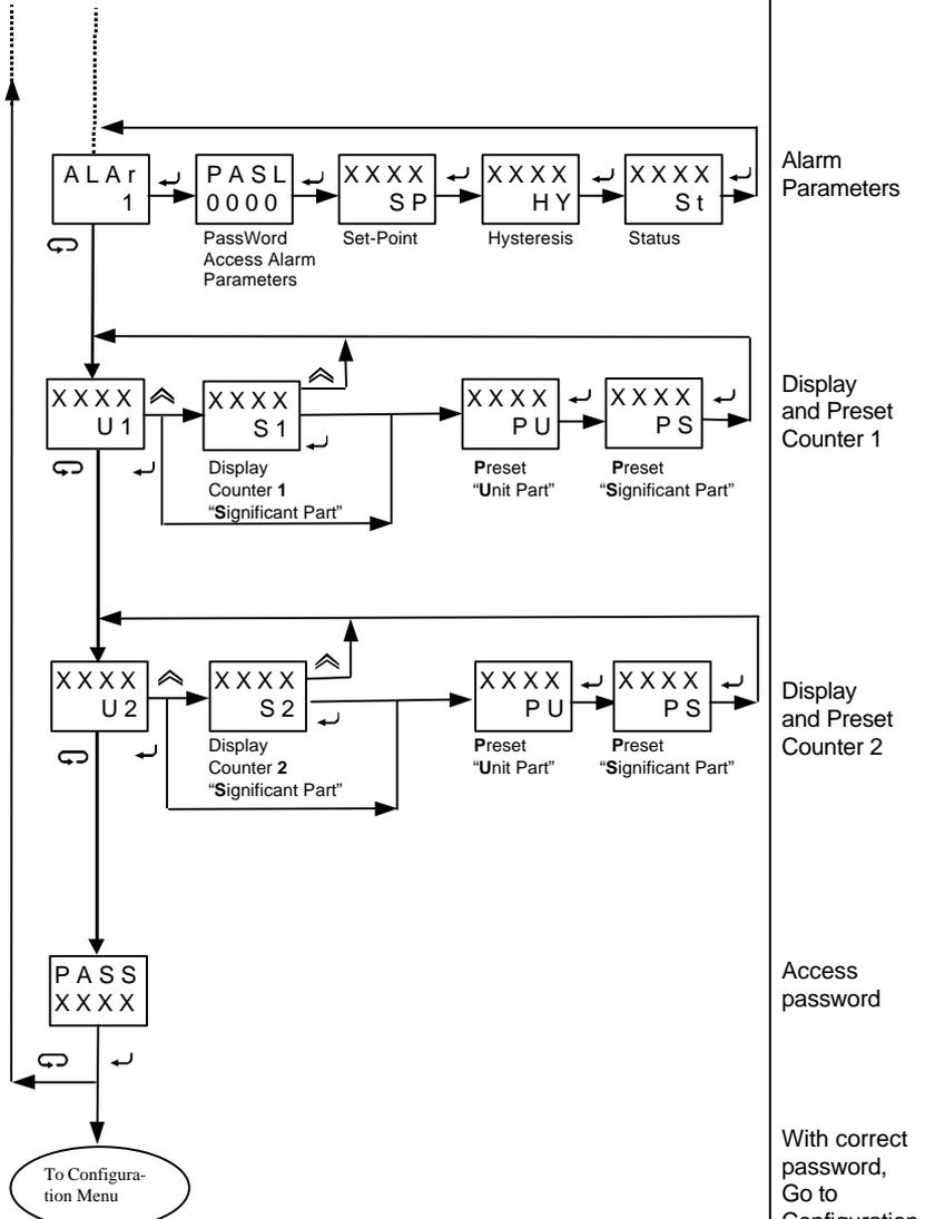
The operation of the Display Menu, is explained in the chapter, "Description of Display Menu Parameters".
