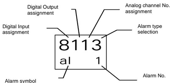
Use the Shift key to select the digit that you wish to modify. Each digit of that code represents an Alarm configuration parameter, with the value of the digit a number that represents one of several possibilities that this parameter can assume.
