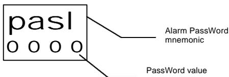
If the password introduced is not correct, the access to the alarm sub-menu is denied. If it has been introduced correctly then will appear the sub-menu to display and/or modify alarm parameters, explained in the following sections.
