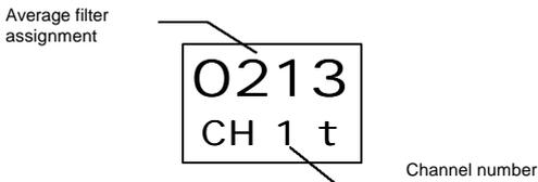
This digit allows you to adjust the Average Filter. This type of filter subdues the abrupt jumps of the measurement signal, performing operations with continued readings to obtain a measurement of more stable behavior than the original signal.
