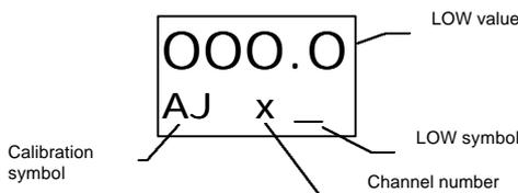
Enter through the terminals corresponding to the number of the channel being calibrated, the signal of the low value: 100 Ohms (0°C of Pt-100).
