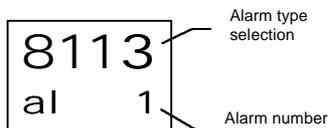
This digit allows you to select the type of alarm activation that the Alarm no. in configuration will have.
