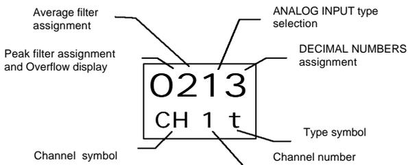
Use the **Shift** key to select the digit that you wish to modify. Each digit of that code represents a configuration parameter of the Analog Channel, with the value of the digit representing the possibilities that this parameter can assume.
