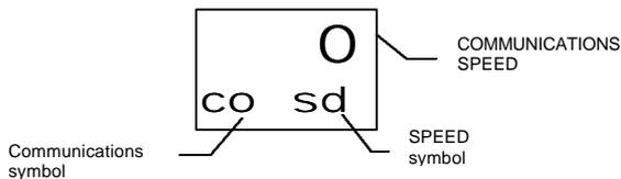
The Communications speed parameter assigned in the last configuration will be displayed. Use the **Increment** key to enter the new value. The possible values are:
