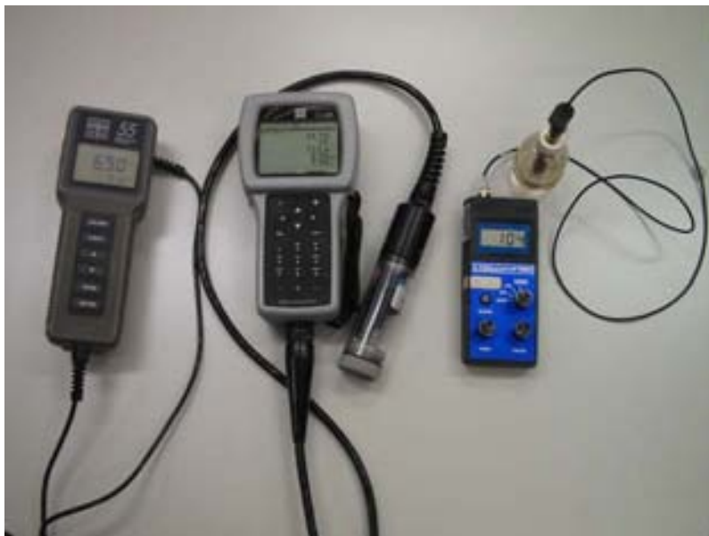
Figure 3 Examples of the various types of field meters available. From left to right: a dissolved oxygen meter, a multi-parameter meter and a redox meter.
