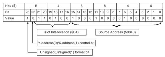
**X/Y Address Bit:** If bit 22 of Ix10 is 0, the PMAC looks for the parallel sensor in its Y address space. This is the standard choice, since all I/O ports map into the Y address space. If this bit is 1, PMAC looks for the parallel sensor in its X address space.
