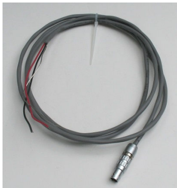
Figure 6. Power Input Cable from Dual Trunk Box
