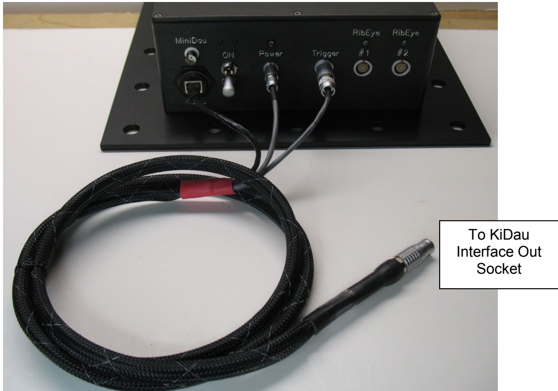
Figure 5. BS-KT-C2 Cable Plugged into Dual Trunk Box
