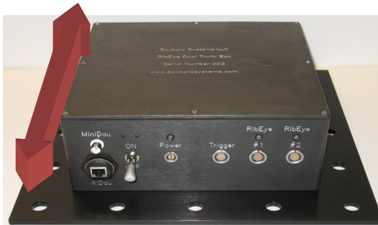
Figure 3. Dual Trunk Box Mounting (Red Arrow Shows Impact Direction)
