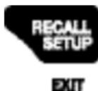
Press this button momentarily to recall or stop viewing logged readings and MIN/MAX readings. Press this button for more than 1 second to start or exit **"SETUP"**.
