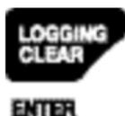
Press this button momentarily to start or stop logging. Press this button for more than 1 second to clear logged readings.
