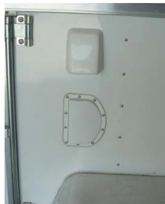
Interior hot air exhaust vent located on the driver's side exterior of the MVSAT-120
