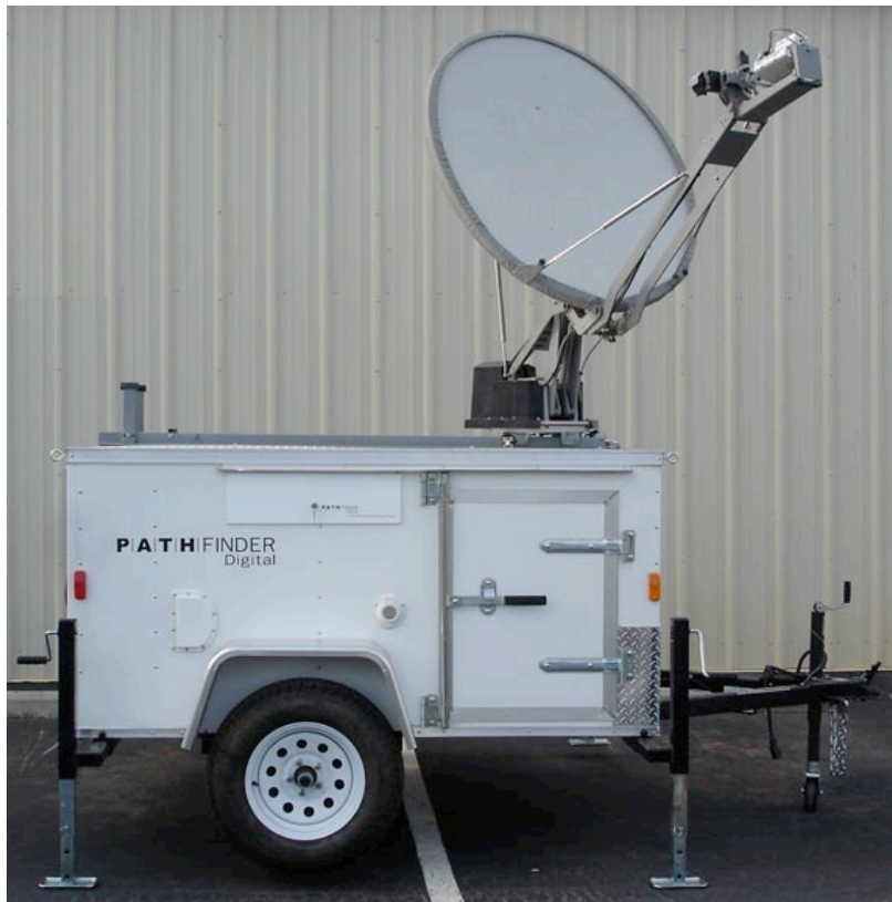
PathFinder MVSAT-120 integrated with the Winegard 1.2 Meter Auto Acquisition Mobile VSAT Antenna System
