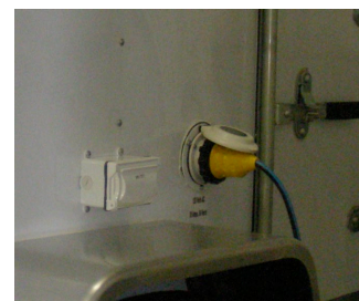
Optional exterior GFI AC power outlet (curbside)
