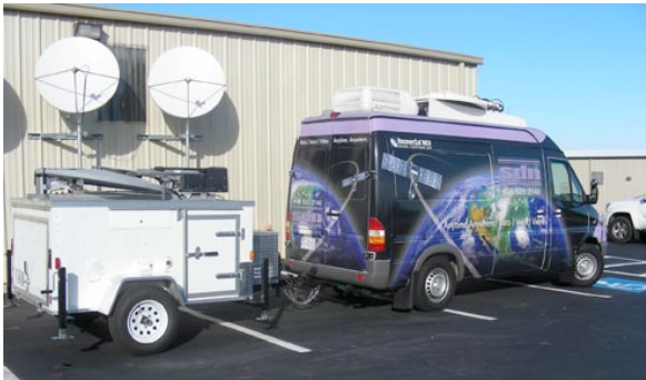
PathFinder MVSAT-120 Transportable SatCom System Trailer Platform integrated with the AvL Technologies 1.2 Meter Auto Acquisition Mobile VSAT Antenna System
