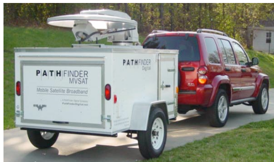
PathFinder MVSAT-120 Transportable SatCom System Trailer Platform integrated with the AvL Technologies 1.2 Meter Auto Acquisition Mobile VSAT Antenna System
