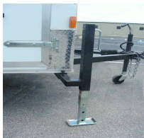
Stabilizer jacks deployed
