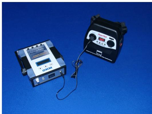
Figure 3: Connection of External Power Supply
