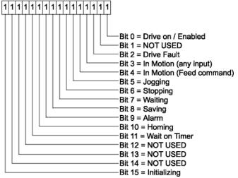
buttons for switching between Hex and Bin (as well as Dec and Oct).
