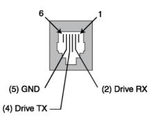
connected to your host's signal ground pin. Pin 4 of the connector should be connected to your host's Rx pin. And Pin 2 of the connector should be connected to your host's Tx pin.
