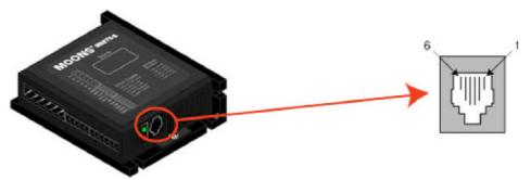
To use SCL in an application means you will have a host device, such as a PC, a PLC, or an HMI, connected to the drive's serial port and using that connection to send commands to the drive. The set of commands defined by SCL includes commands for motion of the step motor, commands for using the three digital inputs, one analog input, and one digital output of the drive, as well as commands for configuring different aspects of the drive like motor current and microstep resolution.
