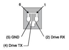
To configure your host to properly communicate with the drive you'll need to configure your host's serial port as follows: 9600 bps, 8 data bits, 1 stop bit, no parity. Not coincidentally, these are the default COM port settings for a Windows-based PC.
