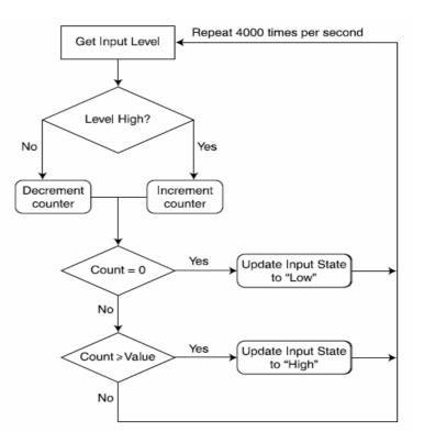
value of 1 equals 250 microseconds. To filter the EN input for 2 milliseconds the value of the FI command would then be 2 msec divided by 250 usec, or 8. The correct syntax for the FI command would then be "FI38".
