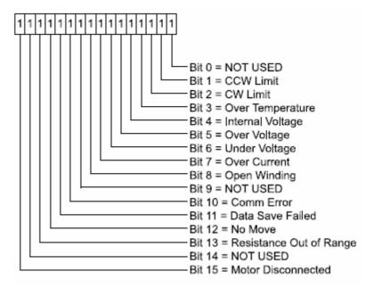
Example: The drive has hit the CW limit (Bit 2), there is an under voltage condition (Bit 6), and an encoder wiring connection has been lost resulting in an encoder fault (Bit 9). The resulting 16-bit word is 000000100100100 - and the equivalent hexadecimal value is 0244. Therefore, when the host sends "AL", the drive will respond with "AL=244".
