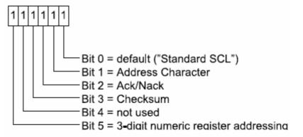
use the PR command the parameter that you send along with the command code (PR) is the decimal equivalent of this binary word. Below are the details of each of the bits and the settings they are assigned to.
