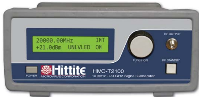
Figure 4: HMC-T2100 Un-calibrated output power indicator
