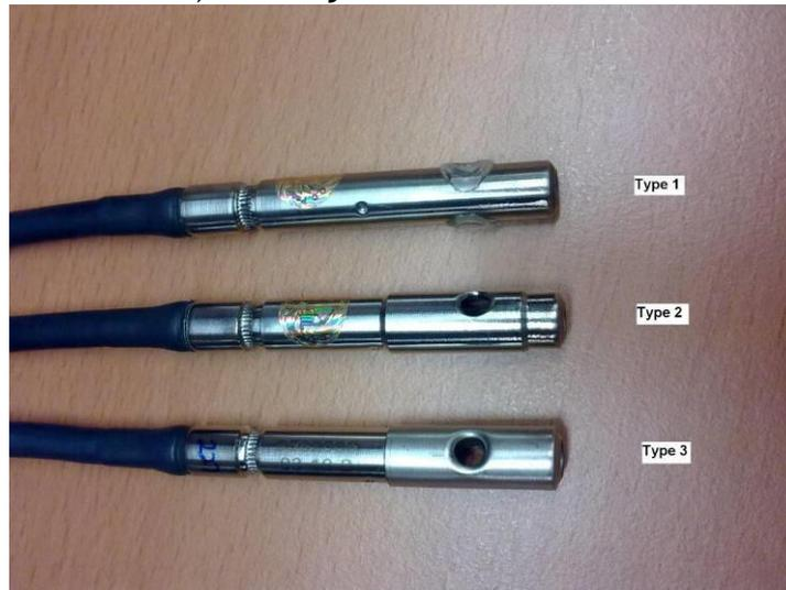
**Type 1** cutters (with plastic inserts) were installed on the first **Vigil® I** (2003 to February 2006) and can be replaced by type 3 at a 40% discount.
