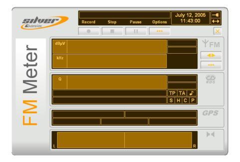
The software is run by means of an RS232C link with the controller from which measurement results will be received.
