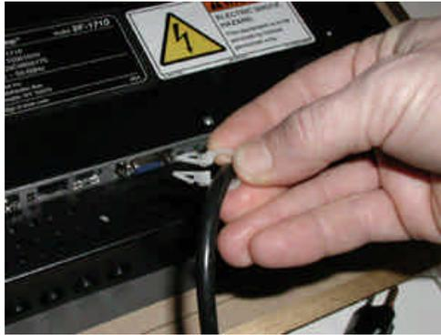
Insert the barb of the clip into one of the four 1/4" holes in the DF-1710's rear housing. These holes are slightly larger than the surrounding ventilation holes. Use one clip for landscape mode:
