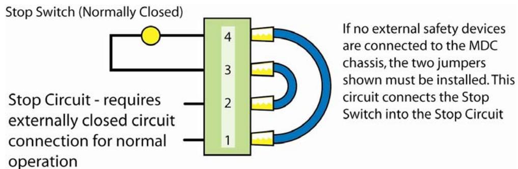
**Figure 5-5: Stop Switch and Stop Loop connections (pins 1, 2, 3 and 4 of Safety Port)**
