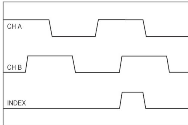
**Figure 6-2: Encoder signal timing diagram for positive motion**
