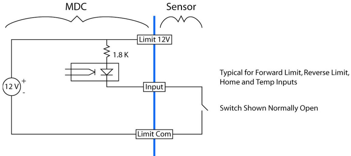
Figure 6-3: Sensor Input Circuit Diagram
