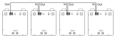
The number of daisy-chained fixtures is limited by the number of DMX channels required by the fixtures in relation to the maximum 512 channels available in one DMX universe. Note that if independent control of a fixture is required, it must have its own DMX channels. Fixtures that are required to behave identically can share the same DMX address and channels. To add more fixtures or groups of fixtures when the above limit is reached, add a DMX universe and another daisy-chained link.
