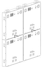
attached side-by-side, and extend the hooks to connect them.
