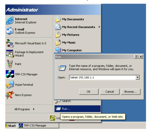
**STEP2.** Click the "OK" TRP-C31S firmware setting will show as following screen. You can set the TRP-C31S by Telnet mode.
