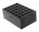
The block at the left is number 620-5013 and is for 30-1.5 ml. centrifuge tubes. The block measures 4.375 in. (11.11 cm.) long by 3.0 in. (7.62 cm.) wide by 1.75 in. (4.45 cm.) thick. All blocks are precision machined from solid aluminum to exactly fit the tube shape and black anodized for better heat transfer and protection from spills. The bottom of the blocks are machined to "nest" on the plate to prevent movement. Also, custom blocks for any sample container can be made upon request.
