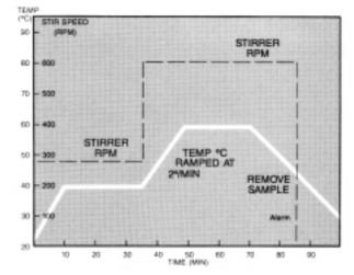
The chart shows a program that can be stored in memory and run at any time. The program can be set to repeat itself from 1 to 98 times, or infinitely.
