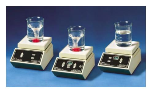
Three models of DigiLog units are available: a hot plate Model HP20, a stirrer Model ST20 and a stirring hot plate Model HS20. All use the same compact, rugged cast aluminum chassis that is designed to keep spills out of the case. All controls are mounted forward of the heater plate for safety. All electronic controls are on one simple PC board, and all controls have red indicator LED's that illuminate when activated.
