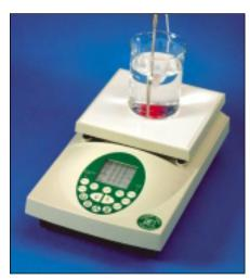
The Model HS40 is fully programmable through the membrane keypad. It can store 10 programs in memory of as many as 10 steps each where a step is a temperature, temperature ramp rate (if wanted), stirring speed and time. Each program can be instructed to repeat from 1 to 98 times. Setting 99 times will repeat the program infinitely. All programs are stored in CMOS. There are no batteries to replace. The HS40 can be used in the programmable and the non-programmable modes.
