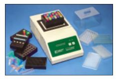
The SC25 is a fully programmable chilling/heating dry bath with builtin orbital mixer. The unit can store 5 programs in memory of as many as 10 steps per program where each step can be a temperature, time and mixing speed. Each program can be repeated from 1 to 99 times automatically.
