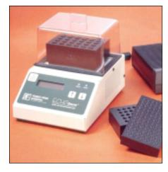
The Model IC25 is the fully programmable version of the IC20. Like the IC20 it does not shake, but it can store 5 programs in memory of as many as 10 steps per program where each program step can be a temperature and time. Each program can be repeated from 1 to 99 times automatically.
