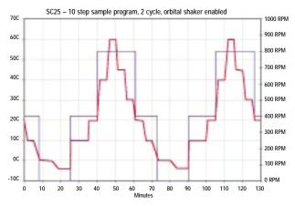
The graph above shows a temperature, time and mixing speed profile that can be stored in memory in the SC25 and rerun at any time.
