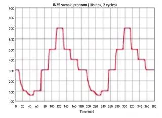
The chart above shows a typical temperature/time profile that can be stored in memory on an IN35 or IN45 and run at any time.
