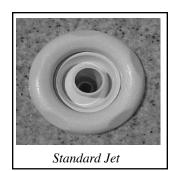
You can adjust both the direction and the velocity of water flow from the Standard Jets. The water flow can be reduced by turning the center nozzle or outer ring (depending on the model) clockwise. By closing one jet, the pressure in the other jets is increased.
