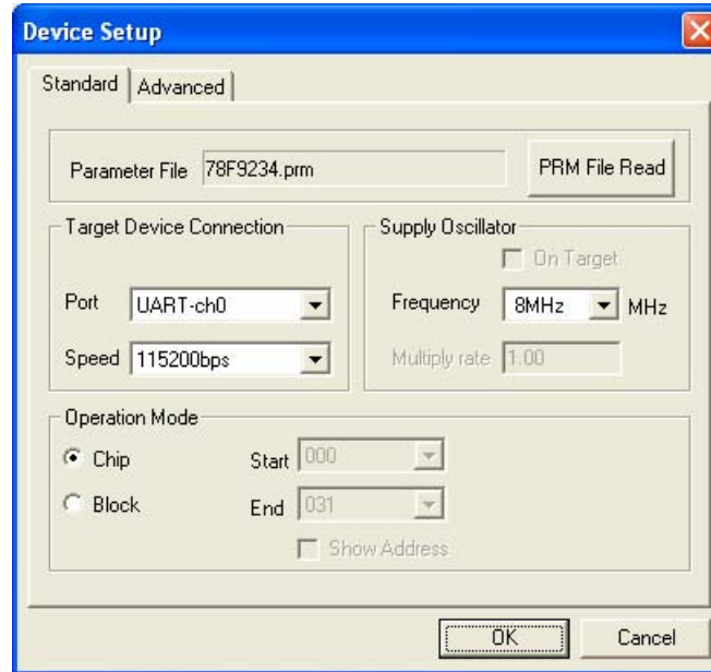
Figure 5-22. [Standard] Tab of Device Setup Dialog Box After Setting
