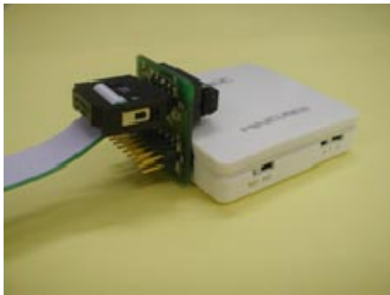
Figure 4-21. With 10-Pin Connector
