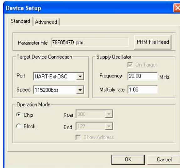
Figure 4-37. [Standard] Tab of Device Setup Dialog Box After Setting
