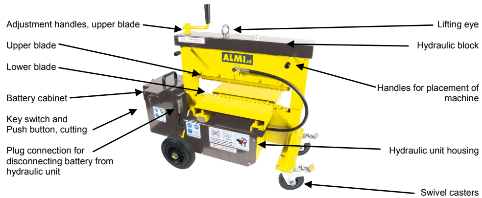
Figure 4.2-1: Construction of the machine
