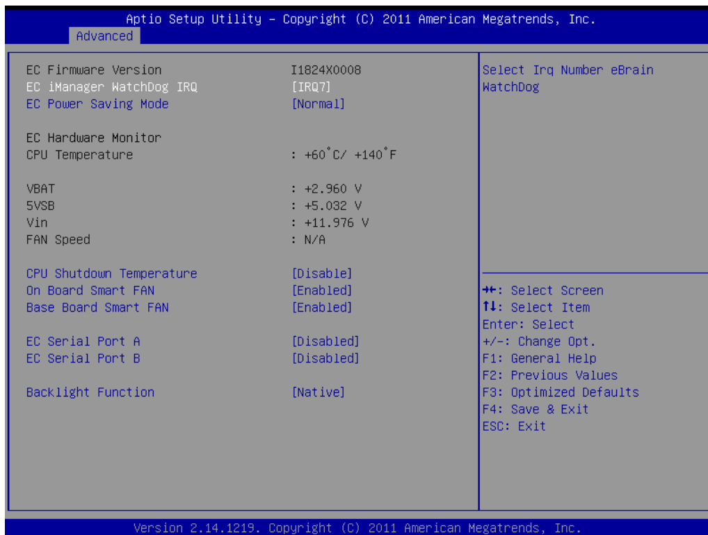
Figure 3.17 Embedded Controller Configuration
