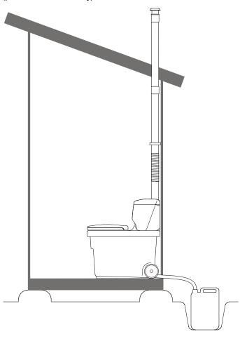
Example of installation with evaporating pan (Picture is indicative only)
